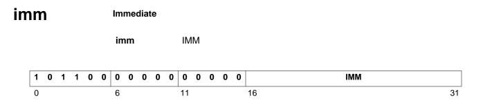
The instruction imm loads the IMM value into a temporary register. It also locks this value so it can be used by the following instruction and form a 32-bit immediate value.
